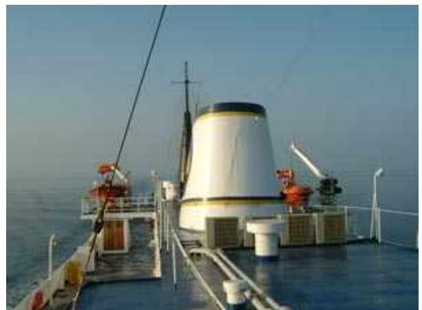
A second fast rescue boat is now carried as can be seen looking aft from the bridge. The MES (marine evacuation slides) have been moved aft to the new open deck from their previous position in the forward lounge. The life rafts shown in the photo on the left are above the new MES position.
